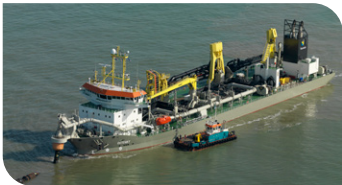
Left: The trailing suction hopper dredger Gateway, which loads up with shingle and then deposits it where needed.
