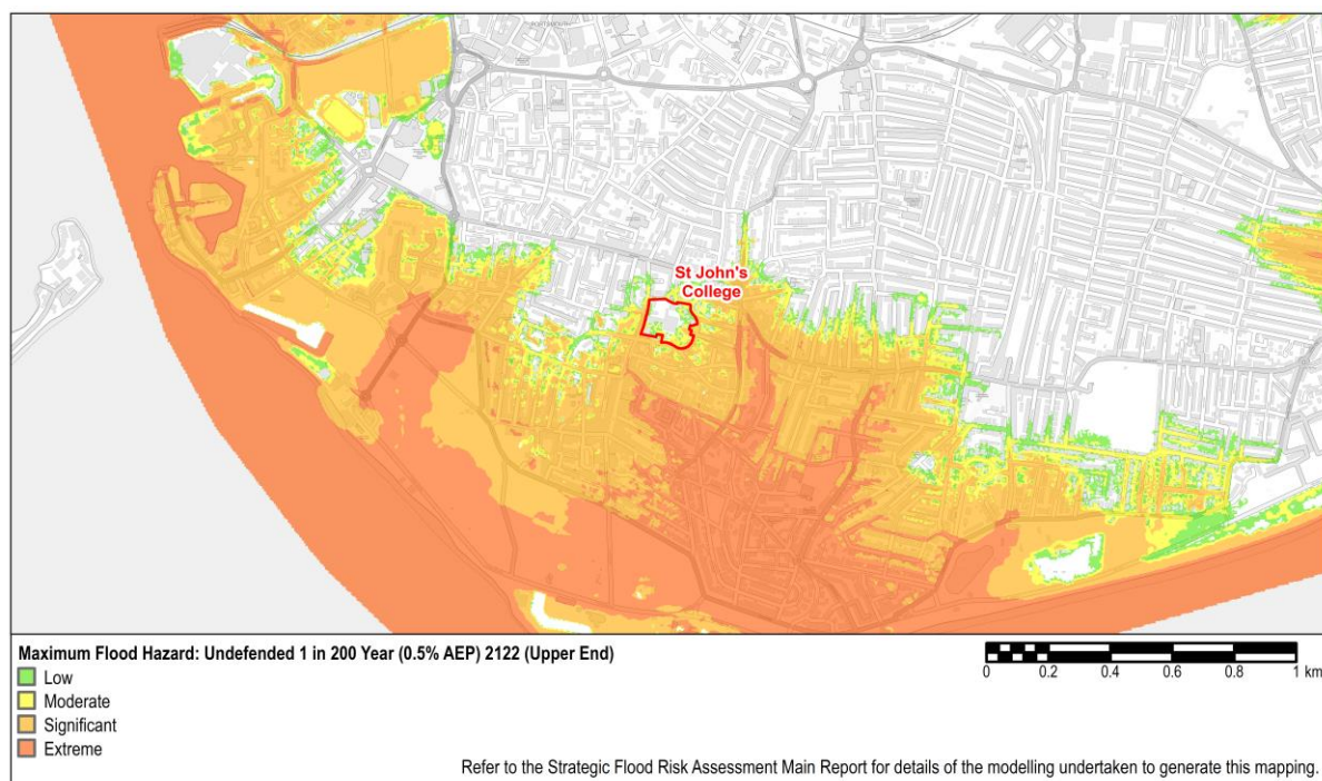
Figure 10-4 Maximum Flood Hazard: Undefended 0.5% AEP 2122 (Upper End)
