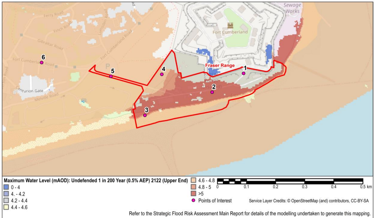
Figure 11-6 Maximum Flood Level: Undefended 0.5% AEP 2122 (Upper End)
