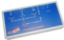
The Epilepsy Monitor is placed under the mattress, analyses the frequency of movement and activates an alarm when appropriate. A microphone is also used to detect sharp gasps, clicks or groans.
