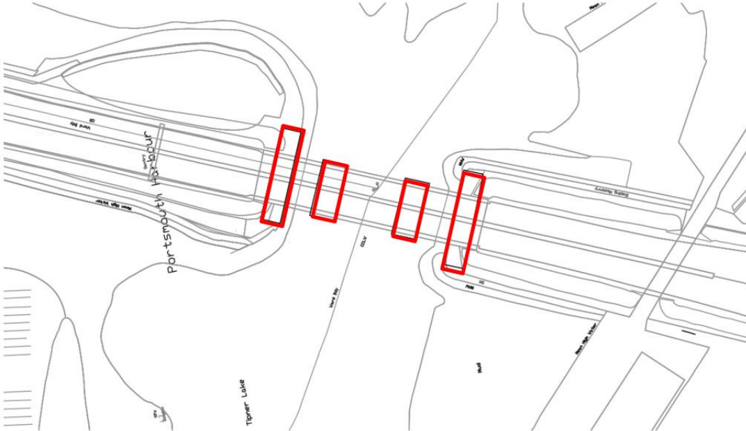
Figure 2 – M275 Bridge Foundations Exclusion Zones
